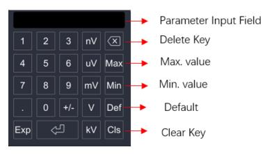
In the numeric keypad, you can use the touch screen function to enter values or units by clicking on them. After entering all numerical values and selecting the desired units, the numeric keypad will automatically close to complete the parameter settings. In addition, after completing the numerical input, you can also directly click the in the numeric keyboard to close it, and the units of the parameters are the default units. In the numeric keypad, you can also perform the following operations:
