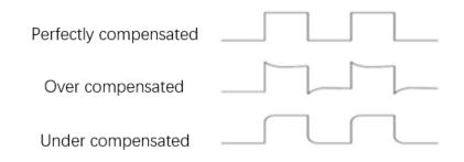
• If necessary, use a non-metallic screwdriver to adjust the variable capacitance on the probe until the waveform displayed on the screen is "Perfectly compensated" as shown in the figure above. If necessary, repeat this step. The adjustment method is shown in the following figure.
